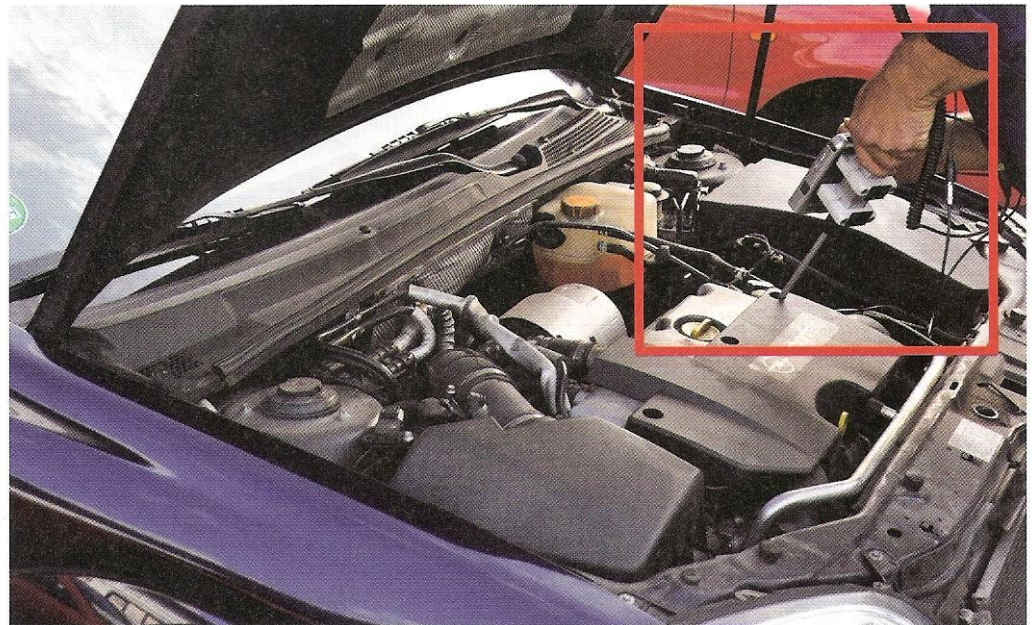
BILD 3: Ultraschallmessung am laufenden Motor FIGURE 3: Ultrasound measurement on running engine
